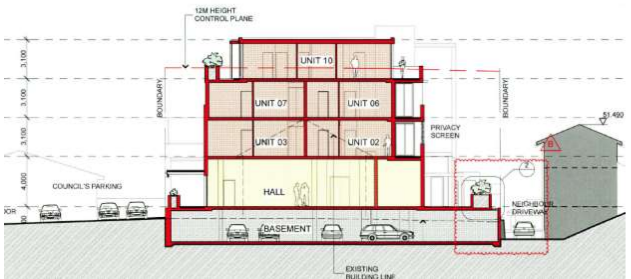
Fig.3 – rear elevation and section
