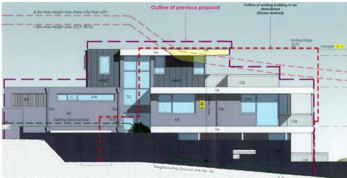
Fig.3 – South-eastern elevation showing non-compliant element shaded yellow.
