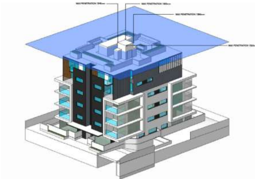
Figure 5: Western view of the areas exceeding the height on the roof level.
