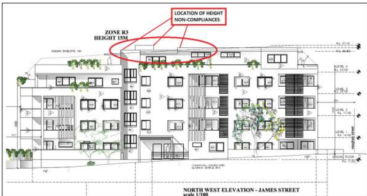
North west elevation, showing location of height non-compliances. Source: Applicant's DA plans, marked up.
