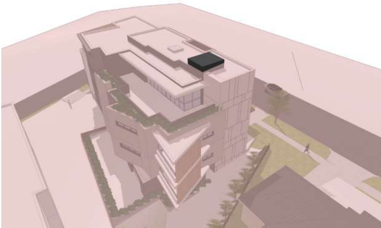
Fig 10. Extracts from applicant demonstrating extent of non-compliance above 12m whereby the upper element of the lift overrun exceeds the height of building.
