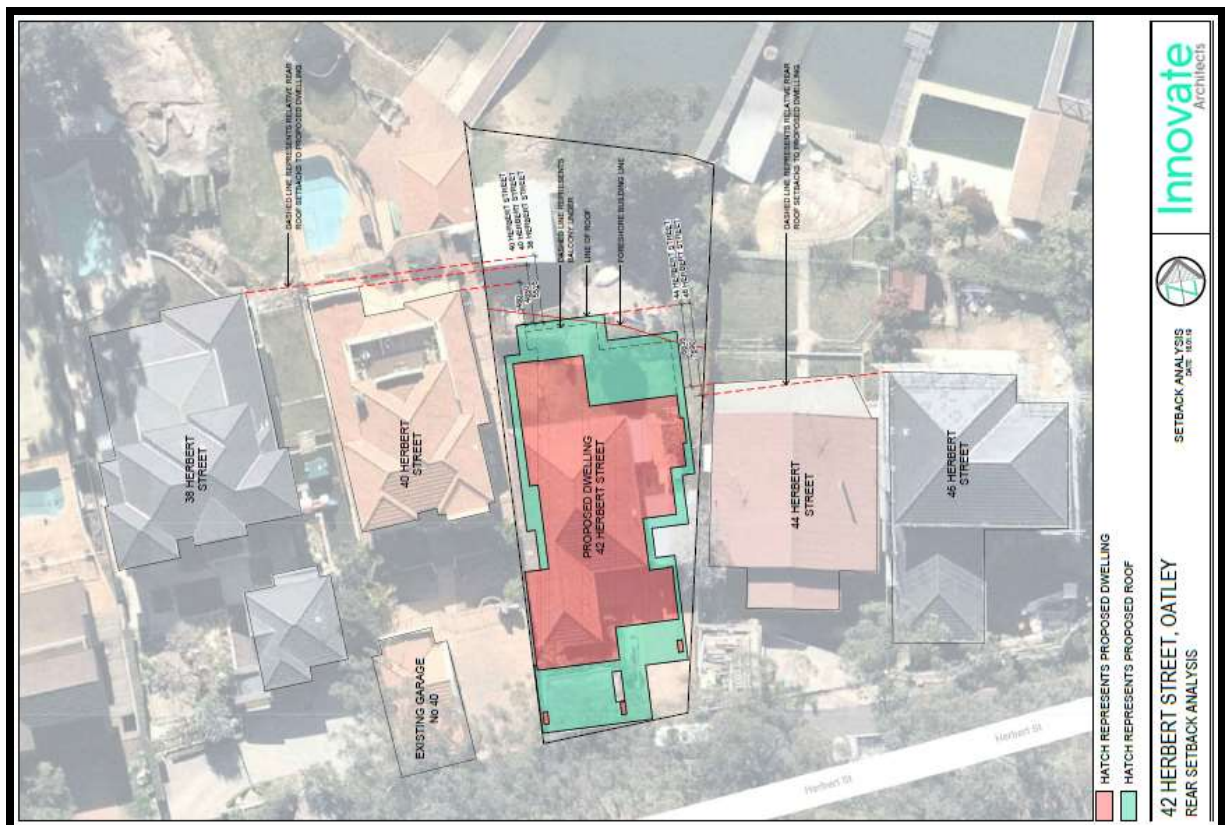
Air photo of subject property showing rear setbacks of the proposed dwelling relative to neighbouring properties
