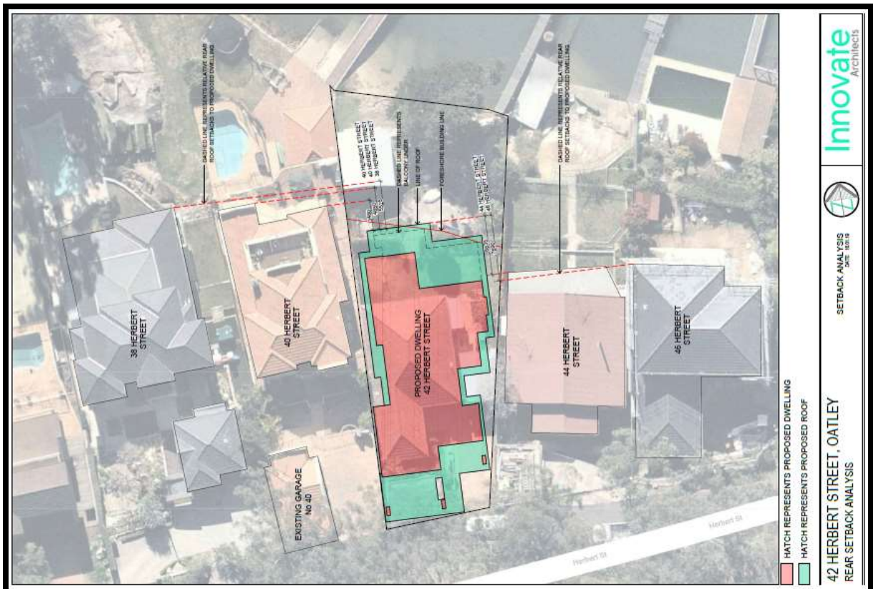
Aerial photo of subject property showing rear setbacks of the proposed dwelling relative to neighbouring properties
