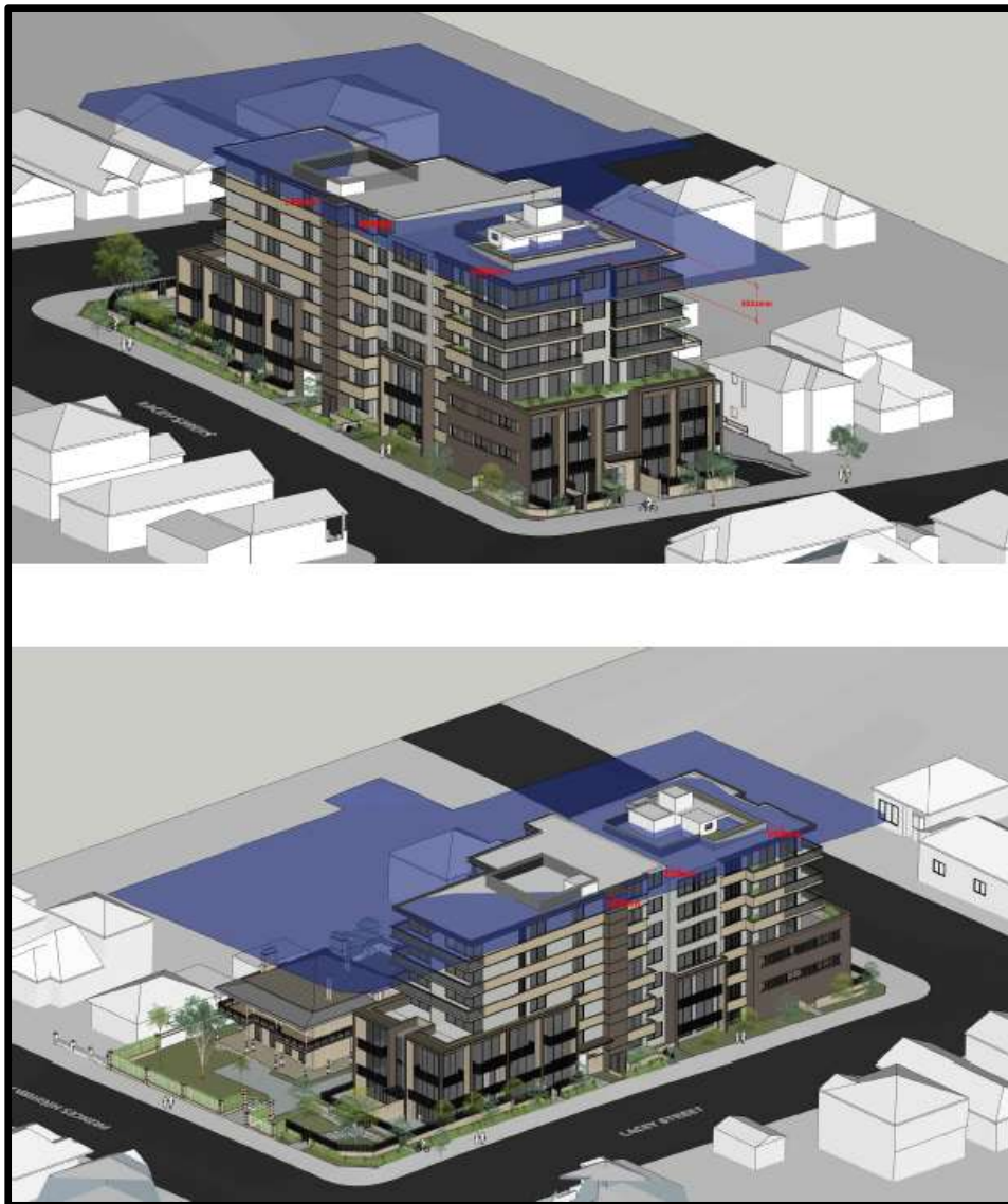
Figure 18: 3D Height diagram showing the sections of the building roof that exceed the height control (courtesy Architects, 2018).
