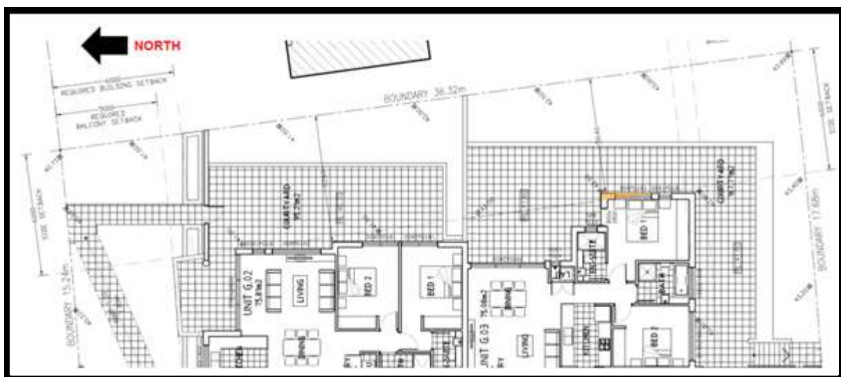
Figure 9: Variation to setback on the eastern elevation.
