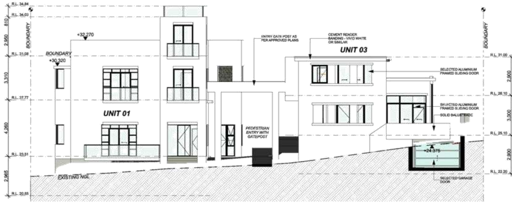
UNIT 1, 3-4 EASTERN ELEVATION 1:100
