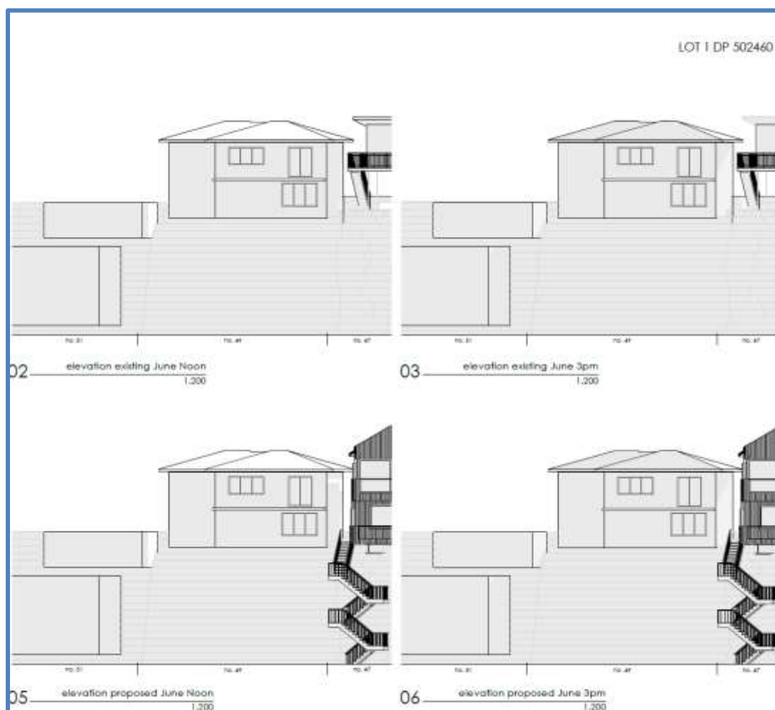
Figure 16: Shadow diagrams in elevation, 12 Noon and 3pm
