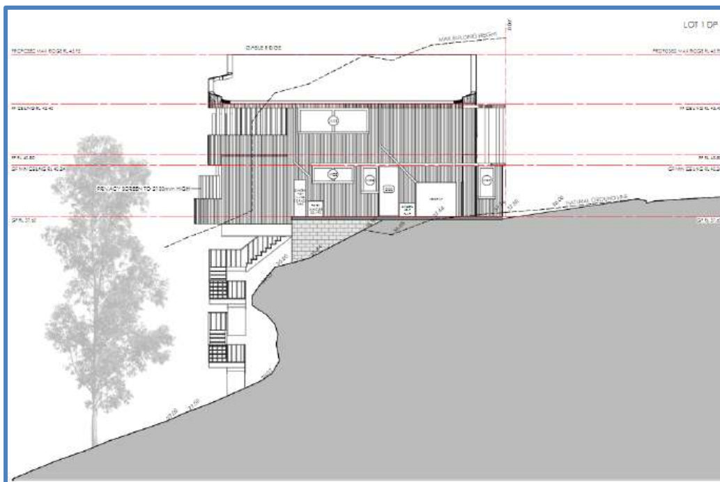
Figure 6: Northern elevation with 9m building height shown dashed.
