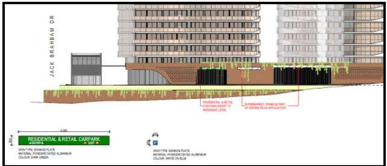
Figure 11: Eastern elevation signage location and detail
