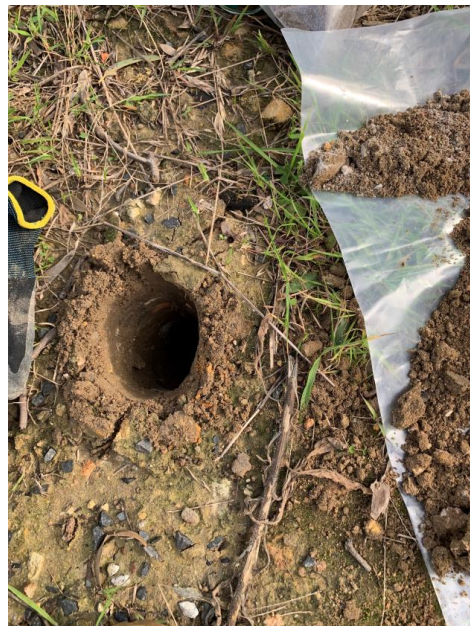
Photograph 14: Typical fill material across the site consisting of gravelly, clayey sand with crushed sandstone, bricks and tiles.
