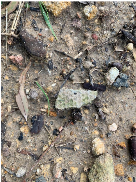
Photograph 13: Suspected Asbestos Containing Material (ACM) fragment on ground surface of fill material in north-western portion of the site .
