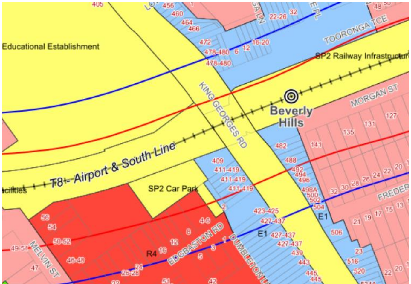
Figure 10 – Location Specific Individual Risk (LSIR) fatality contours for Beverly Hills Local Centre (Source: Draft MSE Pipeline Hazard Analysis Report)
