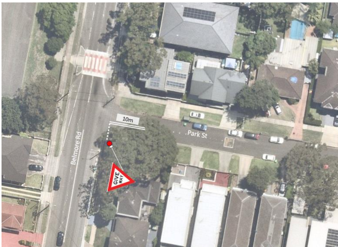
Figure 1 Proposed linemarking and sign at the intersection of Park St and Belmore Rd
