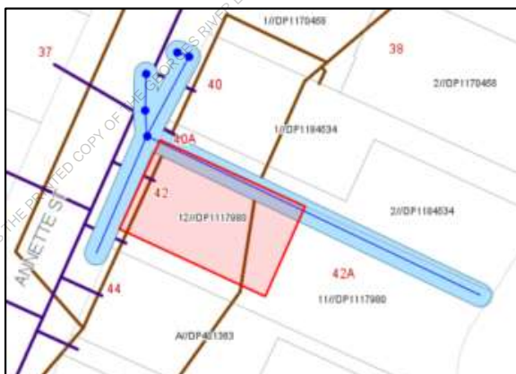
Figure 4 – Sewer mains traversing through front and rear of lot (brown), water connection to lot (purple), Council stormwater main located along northern side boundary (blue) (Source: Intramaps )
