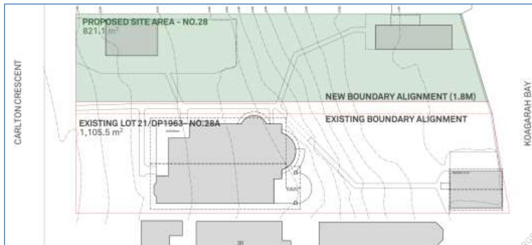
Figure 1: Lot No 22 (28 Carlton Crescent) proposed to be reduced and Lot No 21 proposed to be increased by 114.1sqm (Boundary adjustment plan).
